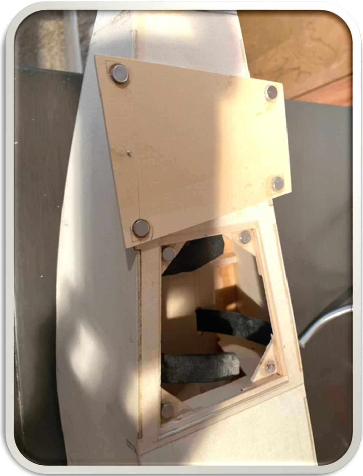
**Closeup of Fred fitting the front hatch with rare earth magnets**
