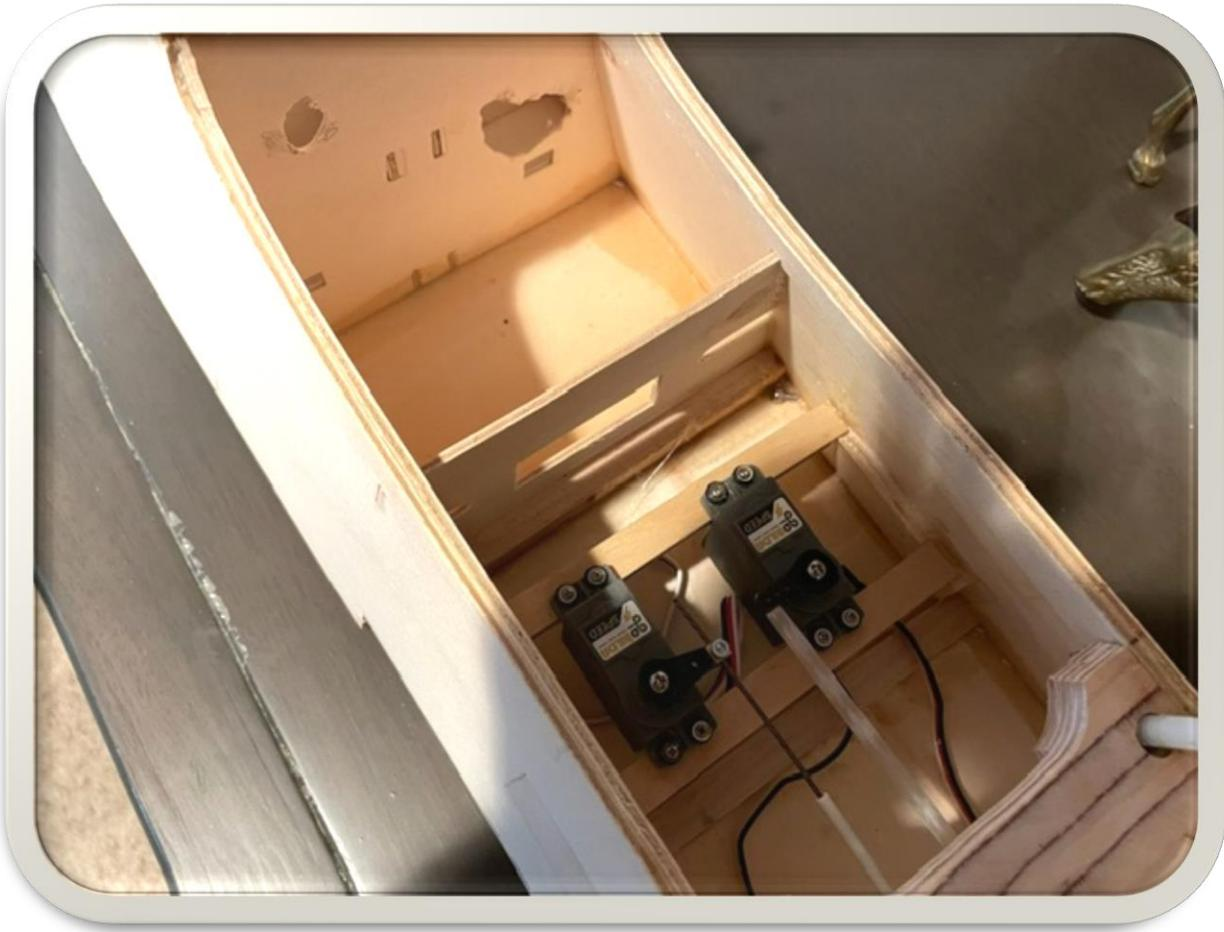
**Closeup of Servo installation in fuselage!**
