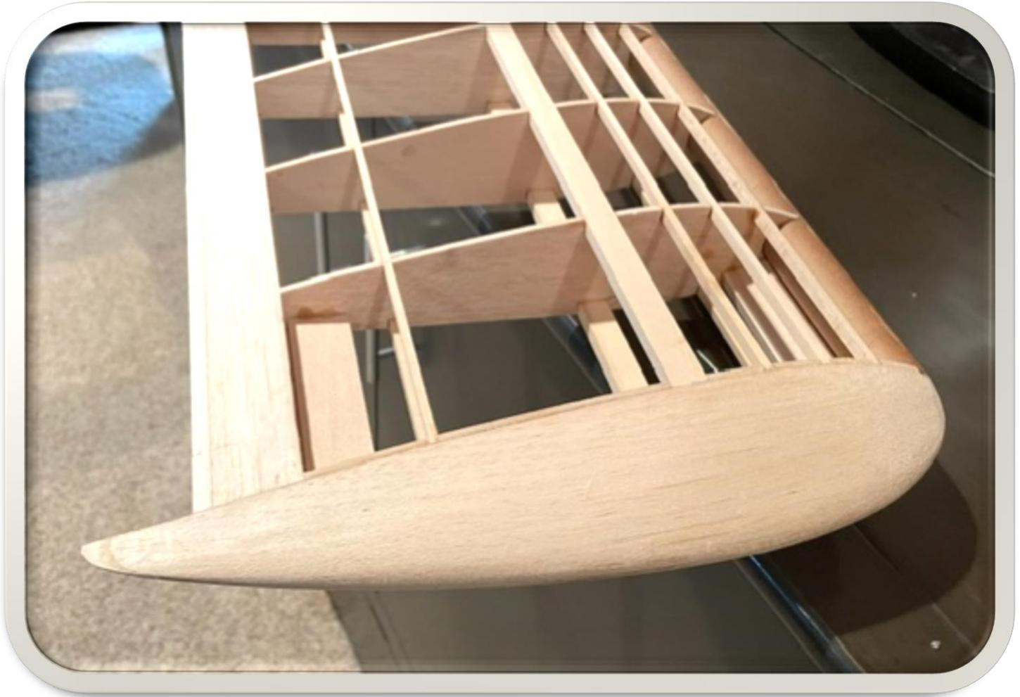
**Closeup of the right wing with ribs, spars minus the ailerons!**
