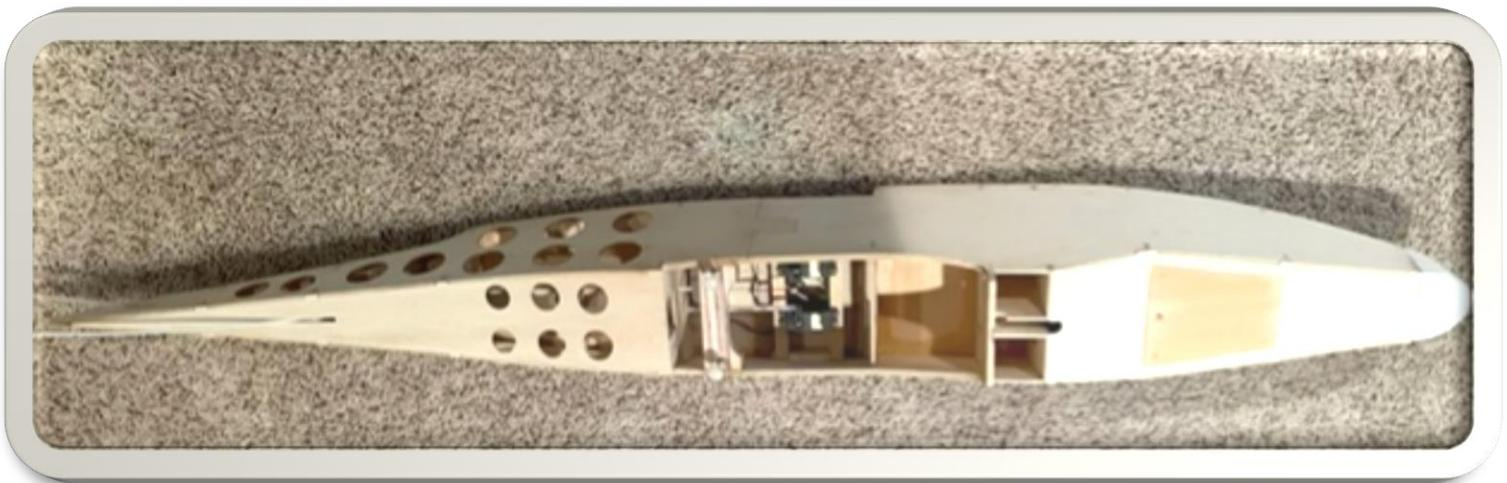
**Top shot of fuselage with Servos fitted!**
