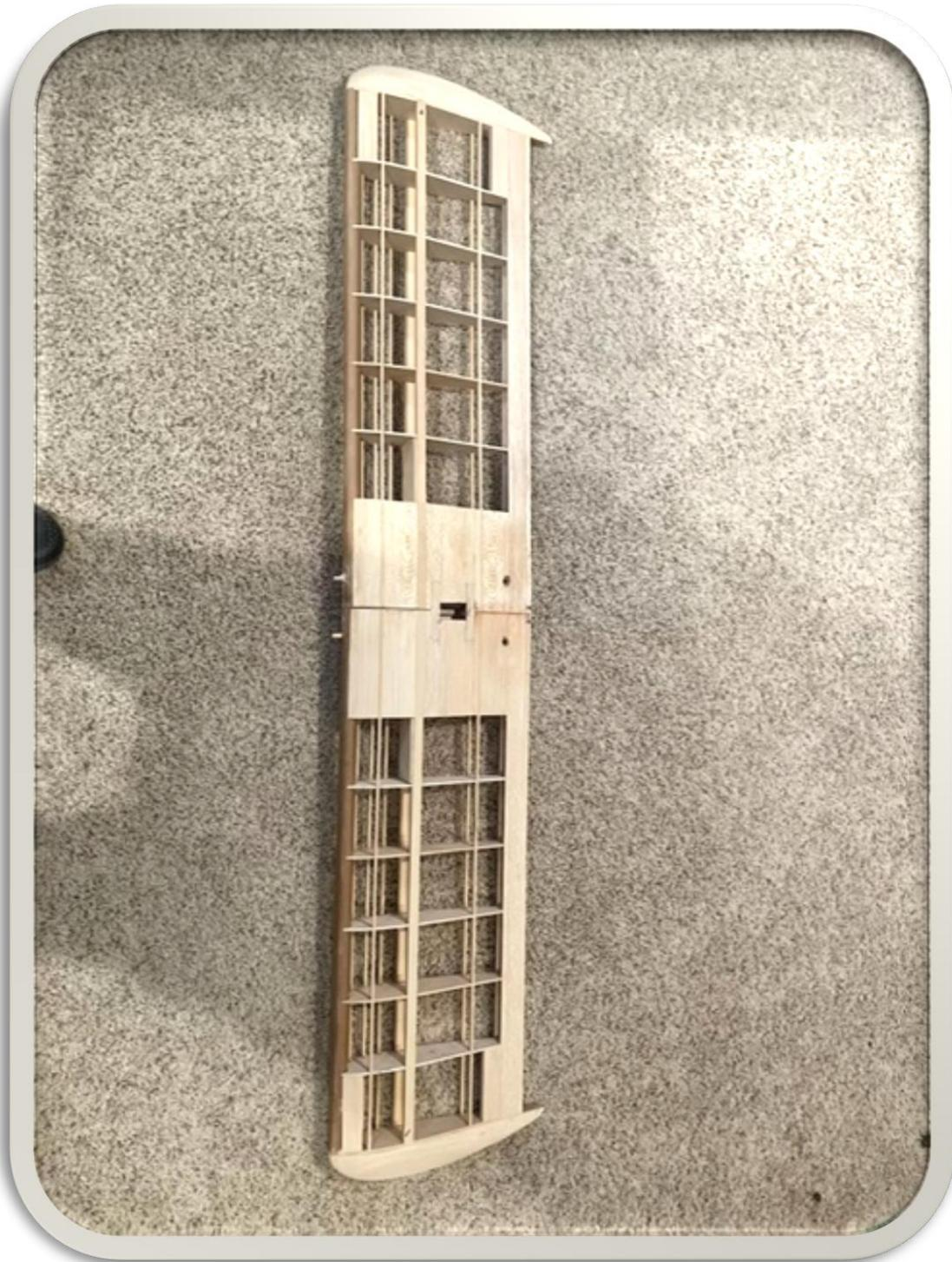
**Full wing with ribs, spars still missing the ailerons! Covering needs to be added.**
