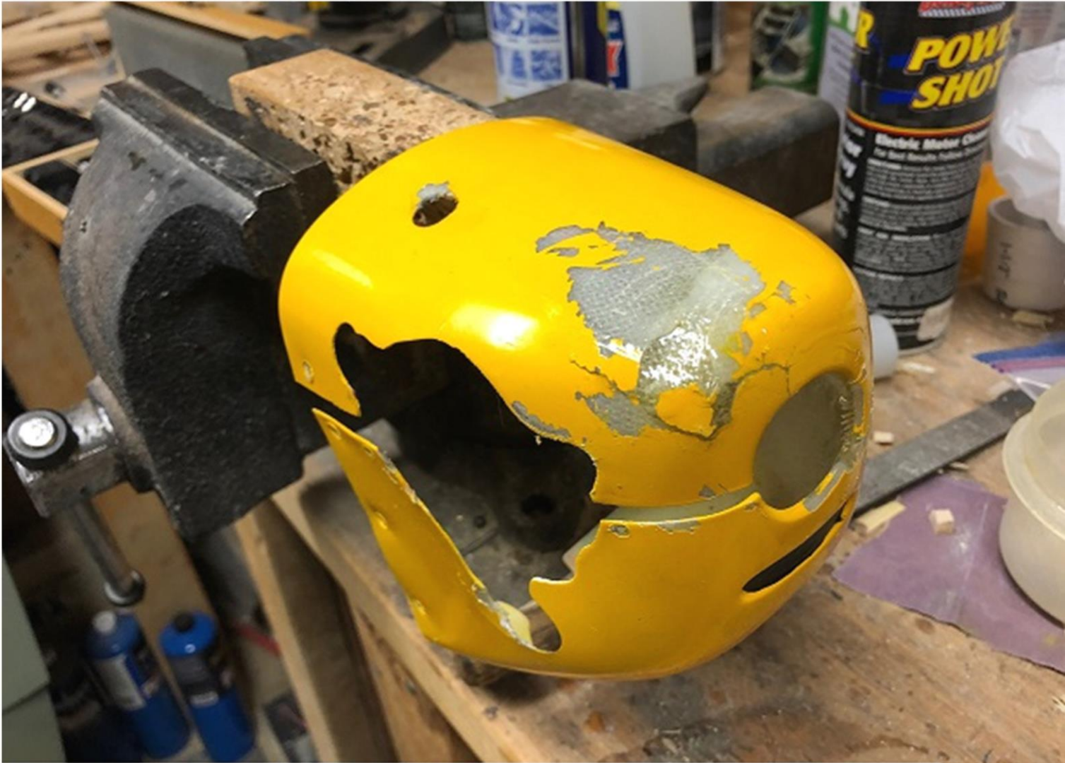
Starting fiber glass repair on cub cowl
