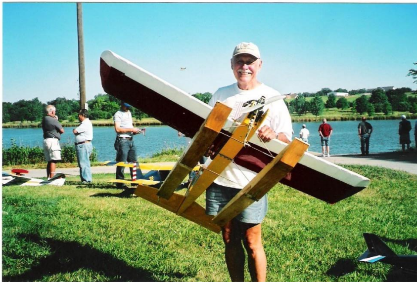
Much used LT 40 with OS 52 FS and Cunningham floats. Floats have thin ply on bottom. Setup has no diagonal bracing, normal landing gear spread & one water rudder. Pilot-Bob Zitzspurger.
