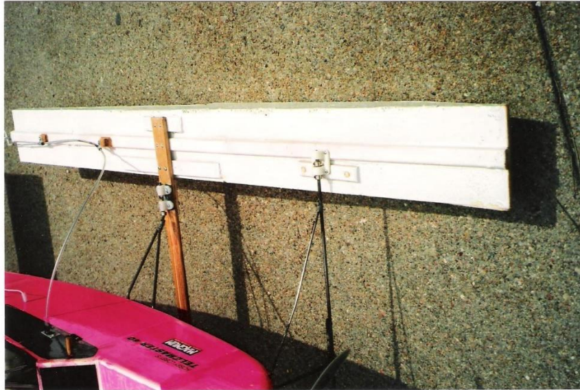
One way to spread and fasten the floats. Setup has diagonal bracing on rear landing gear, laminated hardwood connecting the rear floats and one water rudder.
