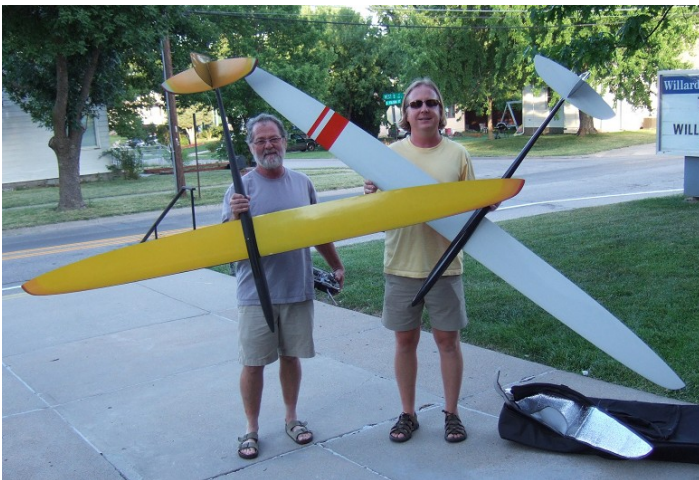
Jim Baker and Thane Kirchoff with their Inertia's (Inertiae?) they brought to at the June meeting. The planes were flown at the Midwest Slope Challenge. The plane is Thane's original design for slope soaring. It uses wingerons for control instead of ailerons and elevator. In the photo below, Jim's plane has a remote-controlled hatch for an airbrake.
