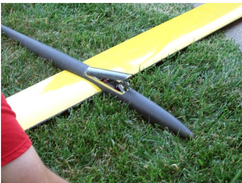
Jim Baker and Thane Kirchoff with their Inertia's (Inertiae?) they brought to at the June meeting. The planes were flown at the Midwest Slope Challenge. The plane is Thane's original design for slope soaring. It uses wingerons for control instead of ailerons and elevator. In the photo below, Jim's plane has a remote-controlled hatch for an airbrake.
