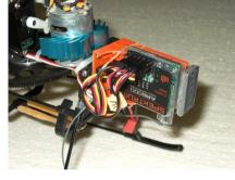
I had a spare 4-in-1 controller. Taking it apart, I found that the receiver was located on one printed circuit board and rest of the electronics were on another. It was a simple task of removing
