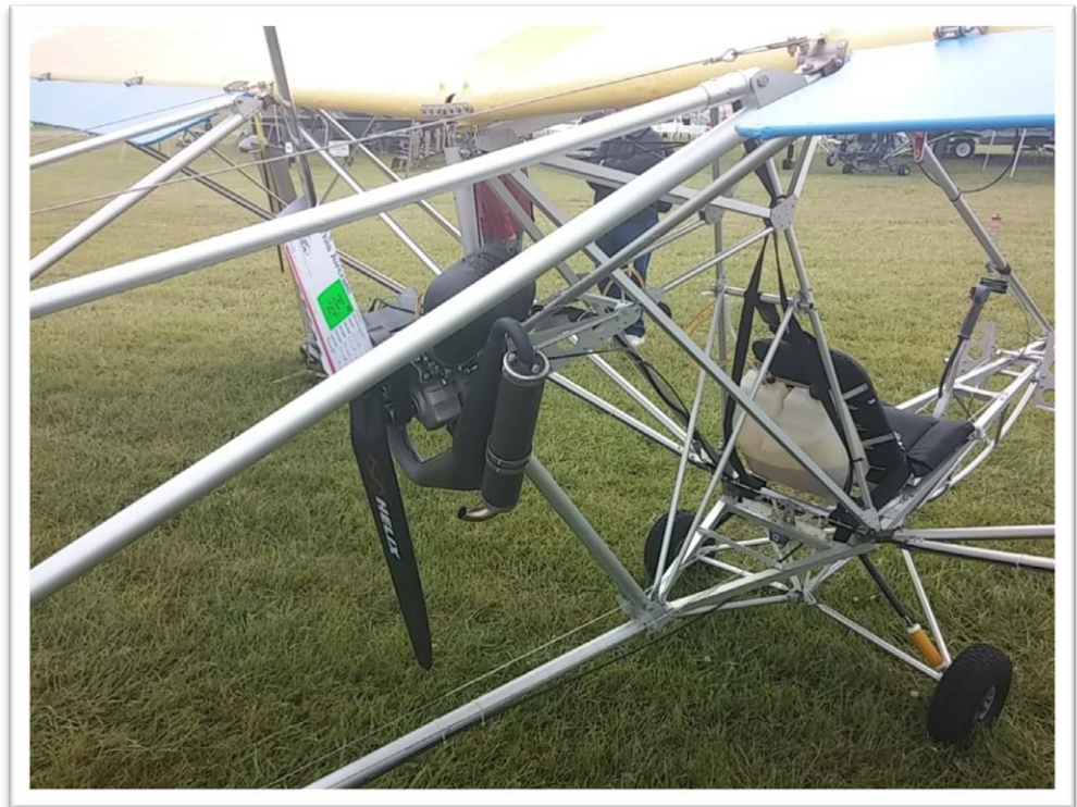
Zigolo uses 25 h.p. Vittorazi PPG engine; can also be electric powered
