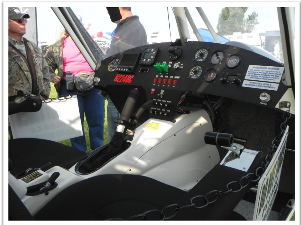
Bush Cat flight deck; each pilot has throttle located in armrest (foldable for entry/ exit)
