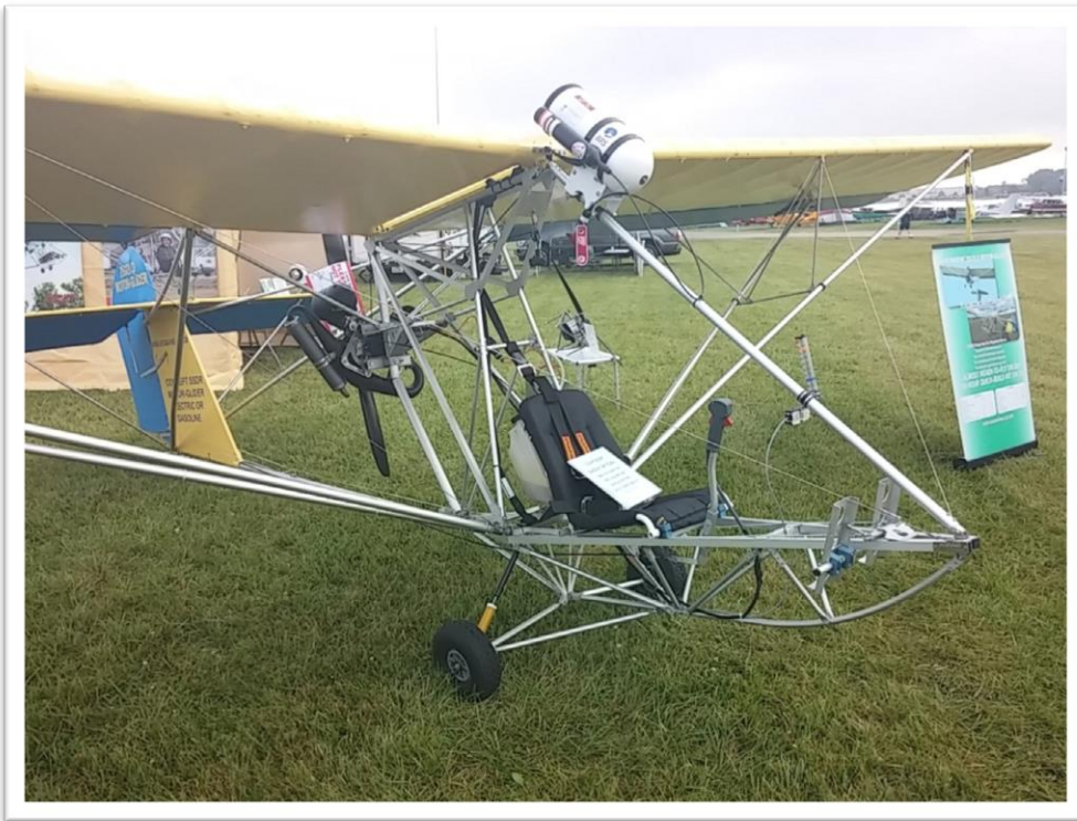
Zigolo uses 25 h.p. Vittorazi PPG engine; can also be electric powered
